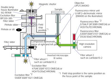
\*2 Use 550DF30 excitation filter in the filter wheel 1 and 575ALP fluorescence filter in the filter wheel 2 when observing red Kaede protein. Exchange of the
