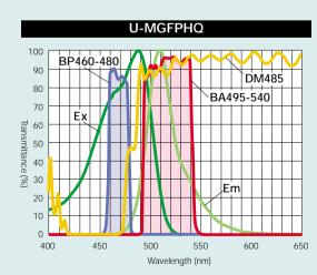
The sharp reactions of the dichromatic mirror in the new mirror unit minimize crossover with the excitation filter and reduce excitation light leakage to less than a tenth of our conventional models. Combined with the light absorbing mechanism (which absorbs more than 99% of stray light), a high S/N ratio is achieved without the need for any special mechanism to prevent excitation light leakage.
