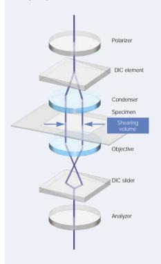
Olympus has developed the most suitable DIC prisms for different types of specimen, based on the shearing amount. When DIC contrast is low, the specimen is hard to observe, while high contrast also hinders observation because of excessive glare. Olympus has therefore developed three different types of DIC prisms to ensure clear observation for every kind of specimen.
